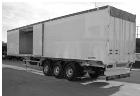
Moving floor with side doors
