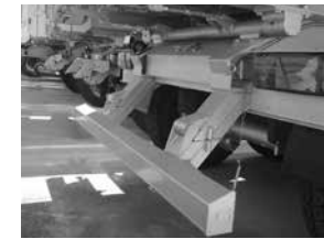
Foldable underride protection
