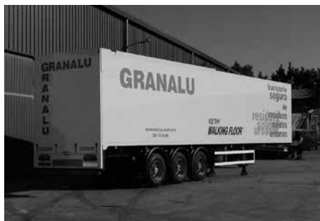
Moving floor for garbage transport
