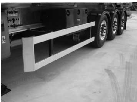
Foldable lateral protection device
