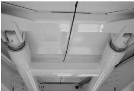
Upper pivot bearing of the undermount cylinder
