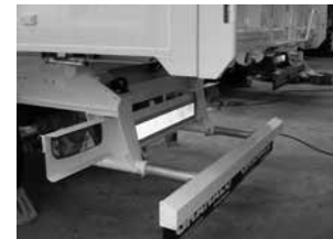
Telescopic underride protection
