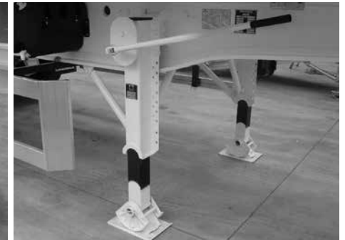
Landing legs out of steel
