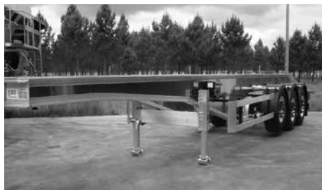
Chassis with an undermount cylinder
