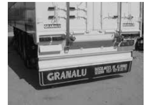
Rigid underride protection
